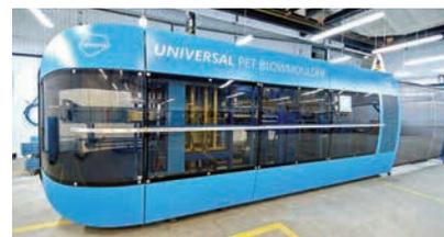
stage PET SBM machine on the market, enabling the production of a wide range of PET containers on one piece of equipment, with necks ranging from 18 up to 110 mm and bottle volumes from 50 up to 6,000 ml.
