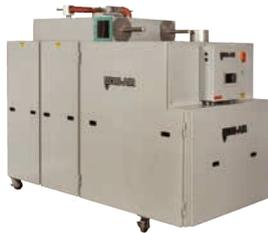
With a compact footprint of 30 square feet, the 1500 FM has a new regeneration air flow design that reduces the previous energy usage level, already one of the industry's lowest, by an additional 25 per cent. And dry air is used for regeneration or cool down of desiccant towers, allowing for dewpoints of  $-26^{\circ}\text{C}$  ( $-80^{\circ}\text{F}$ ) or lower.
